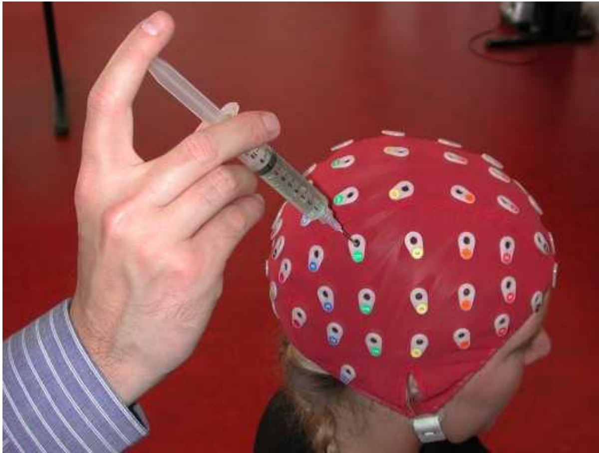
Figure 6.2, depicts orientation of 64 channels elastic cap of the EEG , with the placements of the electrodes using a blunt-tipped syringe, and insertion of the electrolyte gel holes in the cap/sensors;
