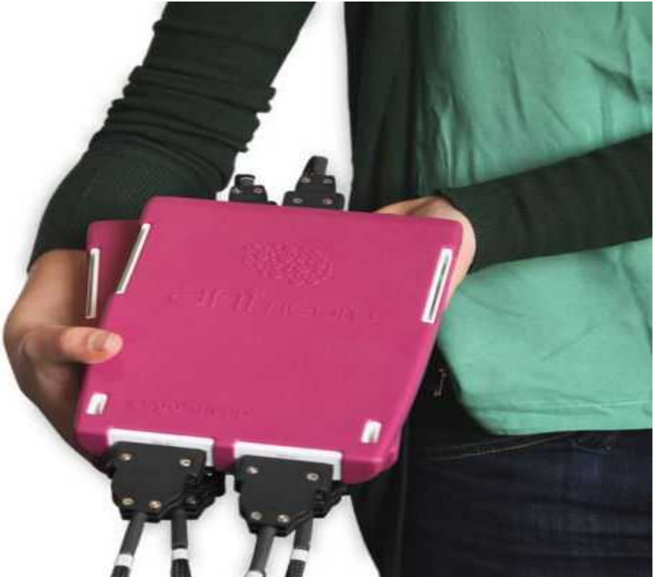
Figure 6.3- depicts the 64-channel Active Two BIOSEMI system (Biosemi, Amsterdam, Netherlands)
